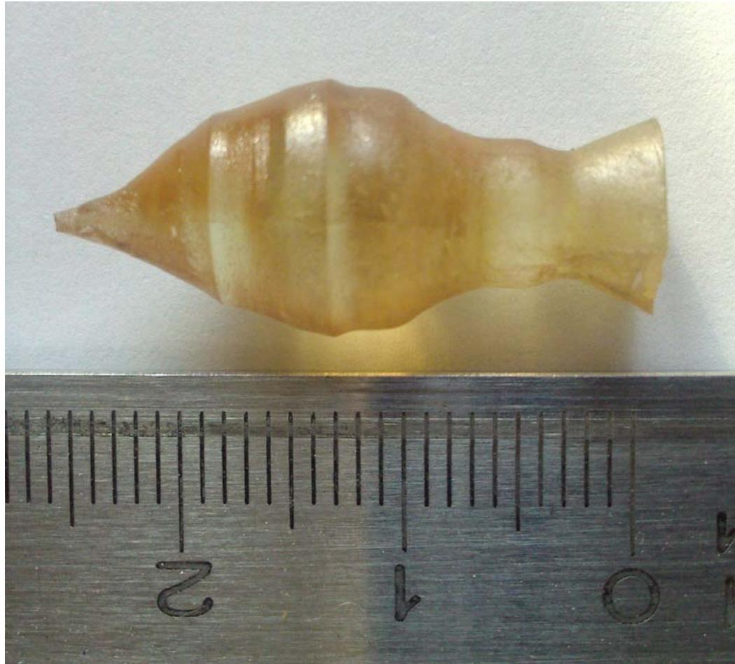
There are no data in literature about crystals of large volume. Fundamental characteristics were measured on very small crystals with dimensions of several millimeters. The main difficulty of crystal growth from the melt is the presence in MgWO<sub>4</sub> crystals of a phase transition below the melting point. For the first time MgWO<sub>4</sub> crystals of ca. >1 cm<sup>3</sup> were grown by pulling the seed from the melted flux solution. .
